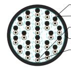
PVC Outer Sheath Tinned Copper Drain Wire Plain Annealed Copper Aluminium/polyester tape XLPE Insulation
